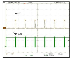
Figure 6. Short-circuit Burst Mode
