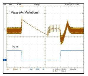
Figure 5. Load Dump from 100% to No-load
