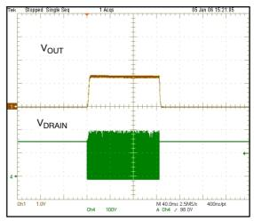
Figure 7. Detail of a Short-circuit Burst
