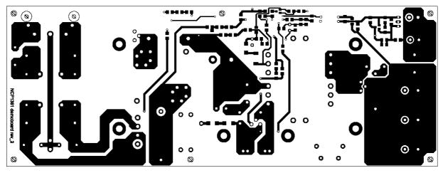
Figure 10. Solder Side (bottom view)
